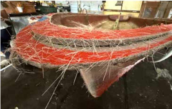
Fiberglass Layers Visible on the first 2027 Flying Scot in Production
